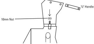
7. Attach the 'U' handle to the hopper sides using the four M8x40 bolts provided (Nyloc nuts inside hopper).
