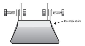
8. A third M8 x 20 bolt plus an 8mm plain washer and an 8mm spring washer have been provided for locking the chute in the operating position. With the chute lowered, place the spring washer then the plain washer onto the bolt, and insert the bolt through the slot at the base of the chute and into the nut that is welded inside the chassis.
