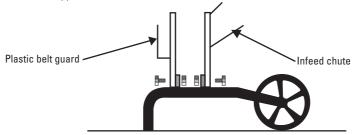
5. Secure the chipper to the base frame using the four 8mm bolts and nuts that were securing it to the pallet.
